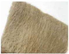
Fig.2. Basalt fiber
